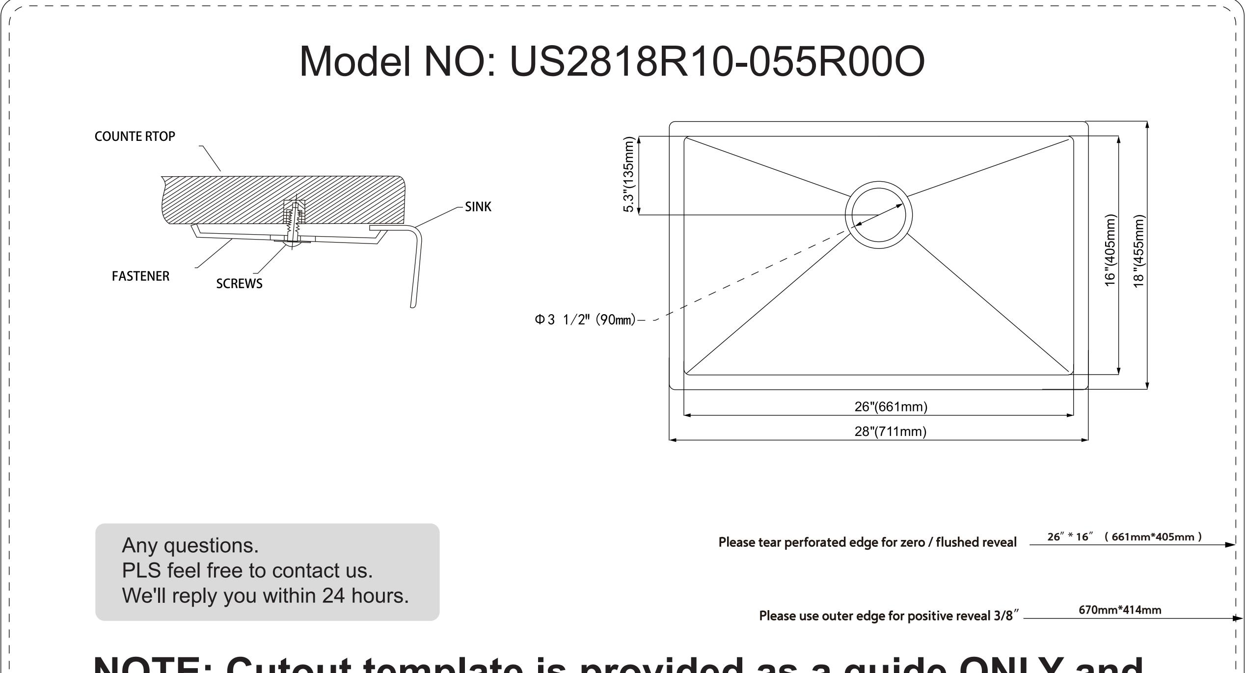
NOTE: Cutout template is provided as a guide ONLY and must be checked against actual sink to verify correct fit.
