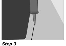
Using a good quality silicone caulk, Apply a generous bead of silicone to the perimeter of the sink's rim.
